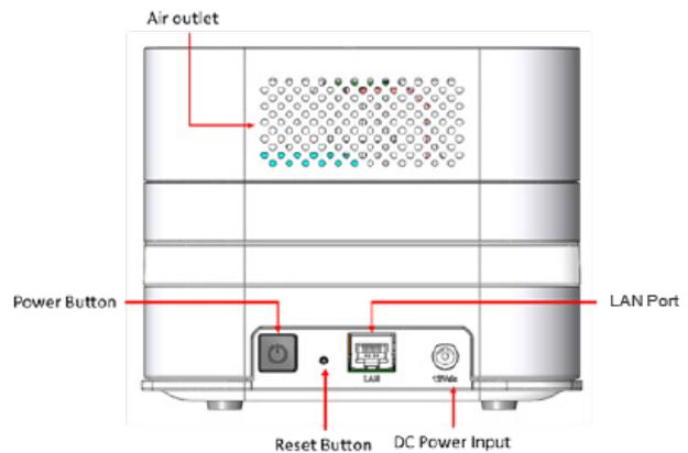
Figure 5: Rear View of the Vetscan Vue+
