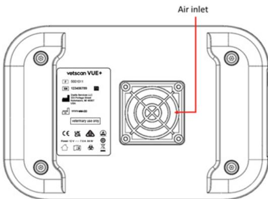
Figure 4: Bottom View of the Vetscan Vue+
