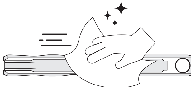
Fig. 18 Wipe Urine Residue from Strip Tray
