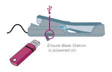
Insert USB drive into the USB port in the Base Station
