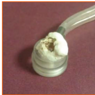
Wash Head with heavy build-up
